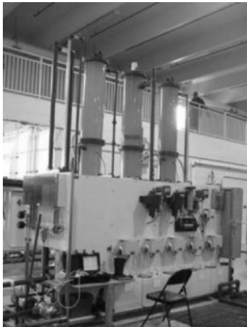
Figure 4. Equipment for media filtration employed at the pilot testing at City of North Miami Beach Norwood WTP (Photograph by Sandeep Sethi 2009, with permission from City of North Miami Beach Utilities, FL)
