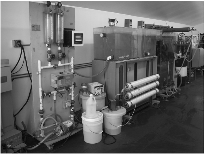
Photo 1. View of Pilot Plant Pre-treatment including Microfiltration (Photograph by Michael Fahy 2006, with permission from El Paso Water Utilities, El Paso, TX)
