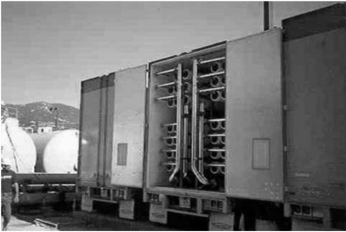
Figure 4. Modular Capacity: One Membrane Trailer (Photograph by Bill Ferguson 2004, with permission from County of Santa Barbara Public Works, CA)
